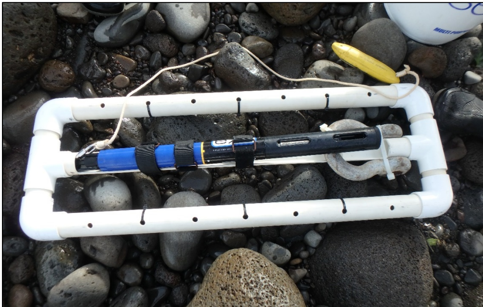
Sonde with weighted frame and attached float.
