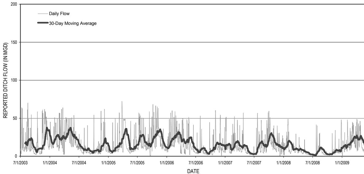
Haiku ditch is the lowest of the four ditches at Honopou. The average ditch flow during this period of record was 6.95 mgd, from a low of 0.05 mgd (June 6, 2008) to a high of 76.53 mgd (March 14, 2004).
