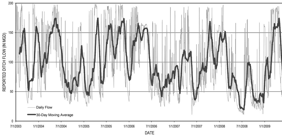
With New Hamakua Ditch located just below Wailoa Ditch for much of its length, the flow drops considerably to an average flow of 18.16 mgd for this period of record. The daily flows for New Hamakua range from 0 to 100.36 mgd (August 16, 2003) with a number of dry days experienced during June and July, 2008.
