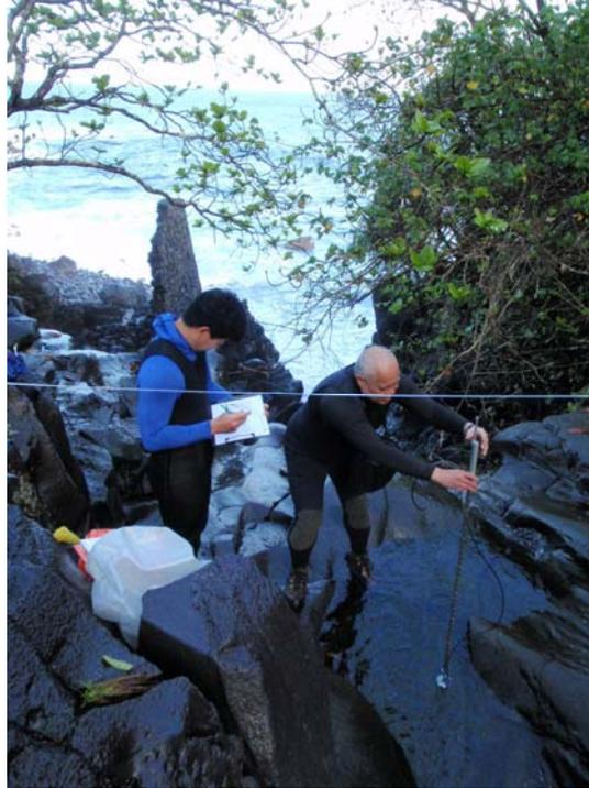
Figure 4-4. Measuring flow at survey site 1, note minimal water flow. Photo taken downstream. (2/9/2009; Tributary name: (64023001), PBN: dk001p-414-020909; Surveyor: Kuamo‘o, D.; Habitat type: Run; SBN: dk001r-020909; Lat. (DD): 20.82704, Long. (DD): -156.09383).
