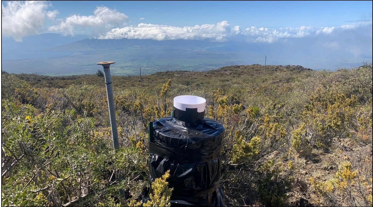
**Figure 5:** A precipitation collector on Haleakalā located near the Haleakalā visitor center at 2,125 m above mean sea level.
